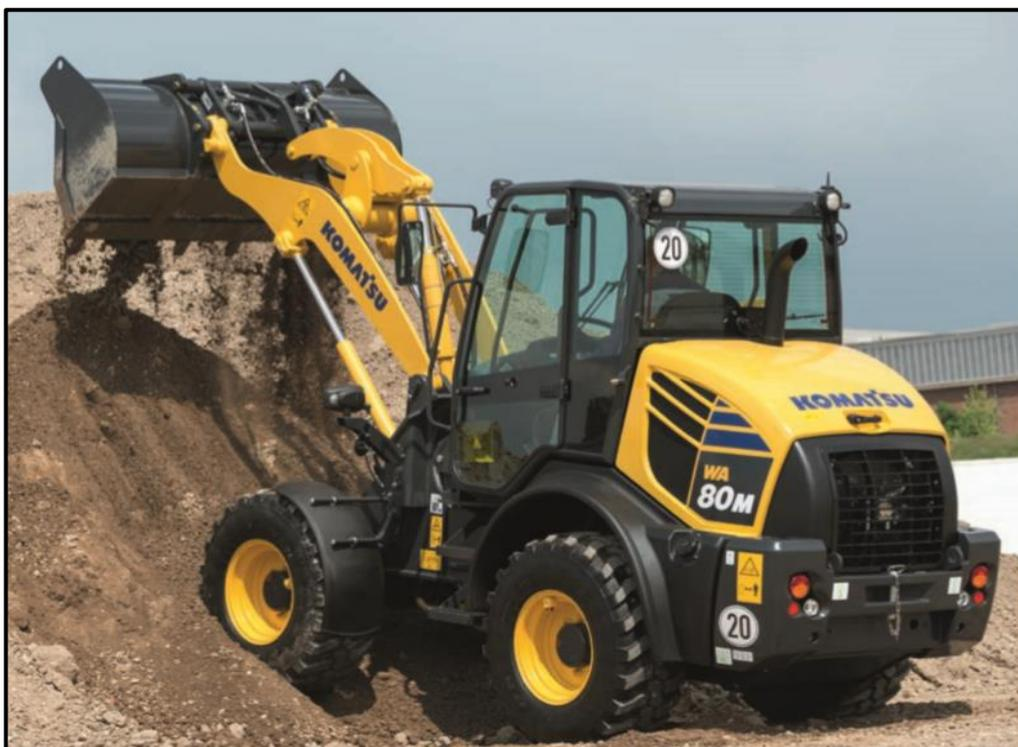
Figura 5.10 Cargador frontal Komatsu WA80M-7
