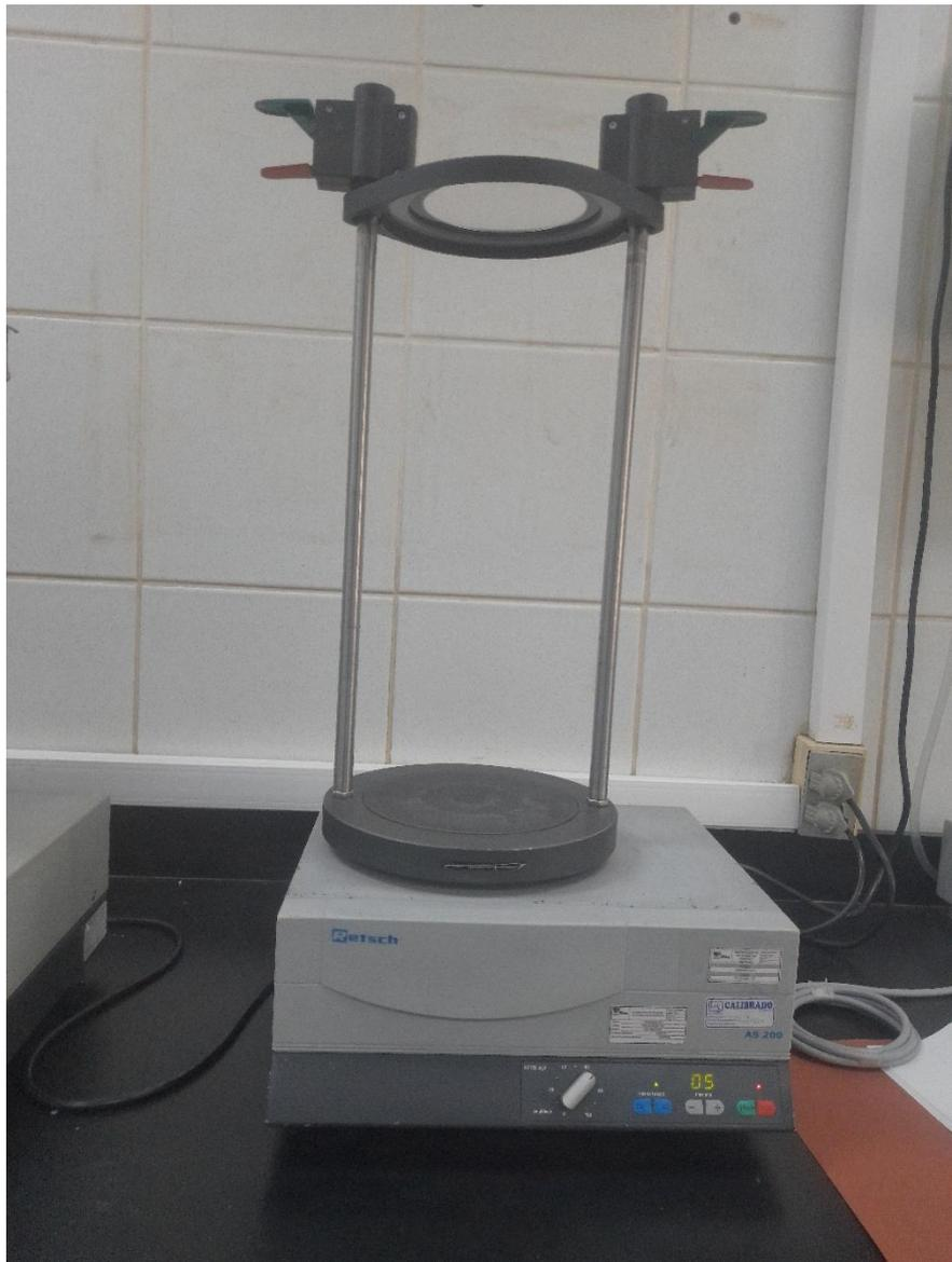
**Figura B.3: Maquina cribadora As 200 digit.**
