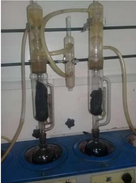
**Figura B.1 Extrator soxhlet**
