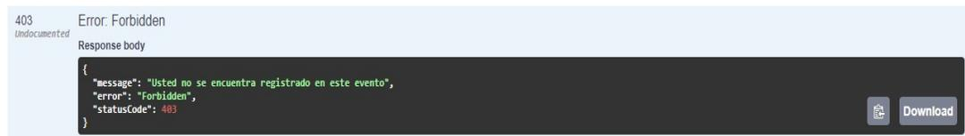
The screenshot shows a light blue header with the text "403 Error: Forbidden" and "Undocumented" below it. Underneath, it says "Response body" and displays a JSON object in a dark-themed code editor. The JSON object contains the following fields: "message" with the value "Usted no se encuentra registrado en este evento", "error" with the value "Forbidden", and "statusCode" with the value 403. To the right of the code editor, there are two buttons: a copy icon and a "Download" button.
